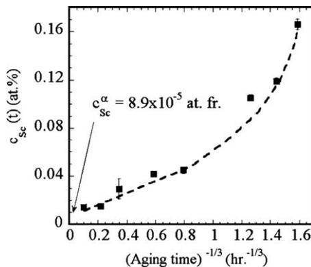
Fig. 7. Scandium concentration in the  $\alpha$ -matrix ( $c_{\text{Sc}}^{\alpha}(t)$ ) as function of (aging time)<sup>-1/3</sup> at 300 °C, yielding equilibrium solid-solubility of Sc in this Al–Mg–Sc alloy,  $c_{\text{Sc}}^{\alpha}(\infty) = 8.9 \times 10^{-5}$  at.fr. The error bars correspond to one standard deviation.
