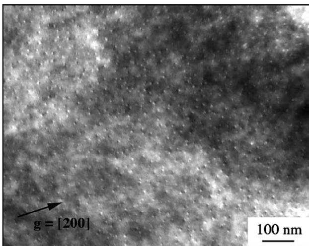
Fig. 2. CTEM micrograph showing a high number density ( $4 \pm 2 \times 10^{22} \text{ m}^{-3}$ ) of  $\text{Al}_3\text{Sc}$  precipitates in an Al–2.2 at.% Mg–0.12 at.% Sc alloy after aging at 300 °C for 24 h: dark-field image, exhibiting Ashby–Brown strain coherency contrast, obtained with a 200 reflection.
