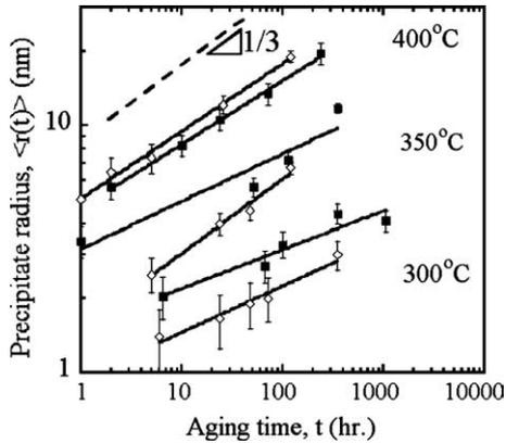
Fig. 5. Log–log plot of the average precipitate radius ( $\langle R(t) \rangle$ ) as function of aging time at 300, 350 and 400 °C in the Al–2.2 Mg–0.12 Sc at.% (filled squares) and the Al–0.18 at.% Sc alloys [3] (open diamonds) versus aging time, yielding the value of the coarsening exponent,  $k_{KV}$ , in Eq. (2). The error bars correspond to one standard deviation.
