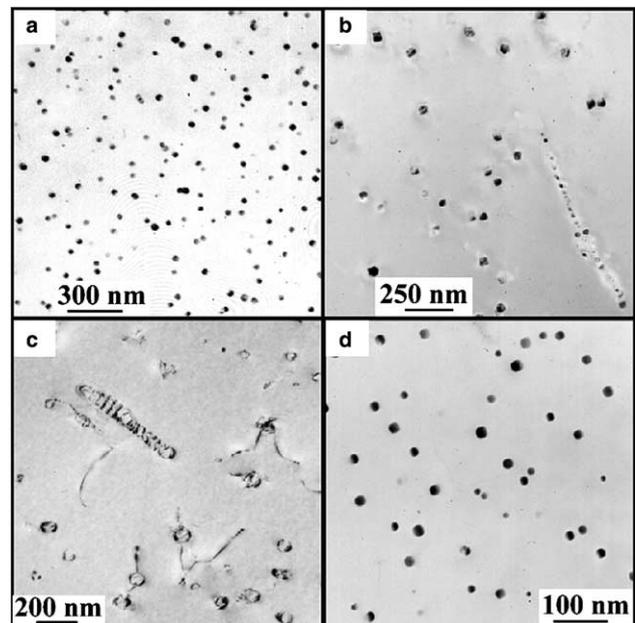
Fig. 4. CTEM micrographs of  $\text{Al}_3\text{Sc}$  precipitates after aging at: (a) 350 °C for 24 h; (b) 400 °C for 2 h; (c) 400 °C for 240 h; (d) 300 °C for 24 h followed by 400 °C for 24 h. The micrographs (a), (c), and (d) are dark-field images obtained using the 100 superlattice reflection.
