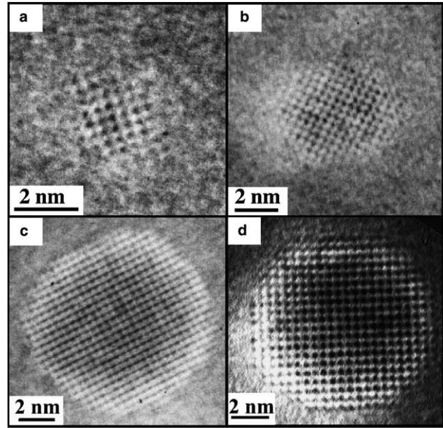
Fig. 3. High-resolution electron microscope images ([100] zone axis) of  $\text{Al}_3\text{Sc}$  precipitates in an Al–2.2 Mg–0.12 Sc at.% alloy after aging at 300 °C for: (a) 0.5 h; (b) 5 h; (c) 1040 h; and (d)  $\text{Al}_3\text{Sc}$  precipitate obtained in an Al–0.18 at.% Sc alloy after aging at 300 °C for 350 h [3].
