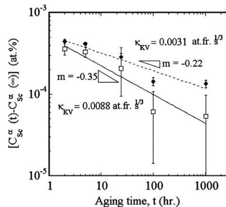
Fig. 8. Log–log plot of the scandium supersaturation in the  $\alpha$ -matrix,  $[(c_{\text{Sc}}^{\alpha}(t) - c_{\text{Sc}}^{\alpha}(\infty)) / c_{\text{Sc}}^{\alpha}(\infty)]$  (at.%) versus aging time ( $t$ ). The empty squares are obtained using our experimental value of the Sc solubility in Al at 300 °C; the filled diamonds are obtained using the Sc solid-solubility data from [7]. The error bars correspond to one standard deviation.
