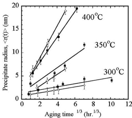
Fig. 6. Mean precipitate radius ( $\langle R(t) \rangle$ ) versus (aging time) $^{1/3}$  ( $t^{1/3}$ ) at 300, 350 or 400 °C (the latter samples were pre-aged at 300 °C for 24 h prior to aging at 400 °C), comparing the coarsening behavior of an Al–0.12 at.% Sc alloy (open diamonds) with an Al–2.2 at.% Mg–0.12 at.% Sc alloy (filled squares). The error bars correspond to one standard deviation.
