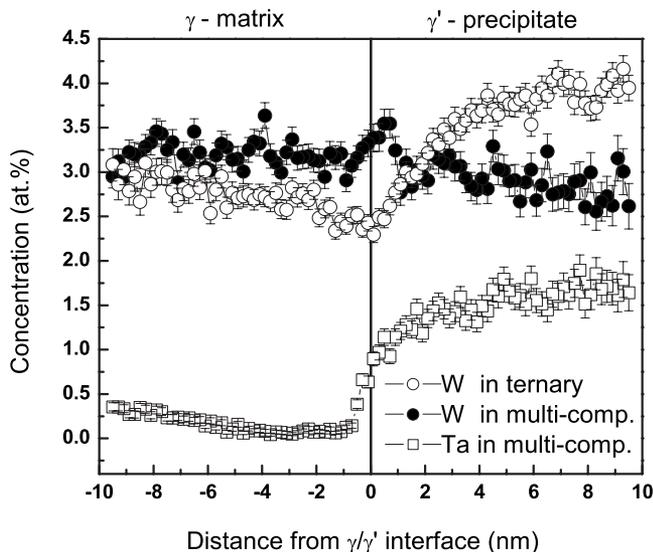
FIG. 2. The experimental APT concentration profiles of W across the  $\gamma/\gamma'$  interfaces of the ternary Ni-Al-W alloy (empty circles) and the multicomponent alloy (full circles). For comparison, the Ta concentration profile in the multicomponent alloy is plotted as empty squares. All profiles are plotted with respect to the isoconcentration surfaces shown in Fig. 1.
