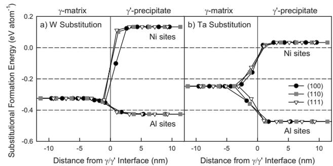
FIG. 3. The substitutional formation energies of (a) W and (b) Ta atoms as a function of the distance from the {100}, {110}, and {111}  $\gamma/\gamma'$  interfaces, obtained using first-principles calculations performed in a model Ni( $\gamma$ )/Ni<sub>3</sub>Al( $\gamma'$ ) system.
