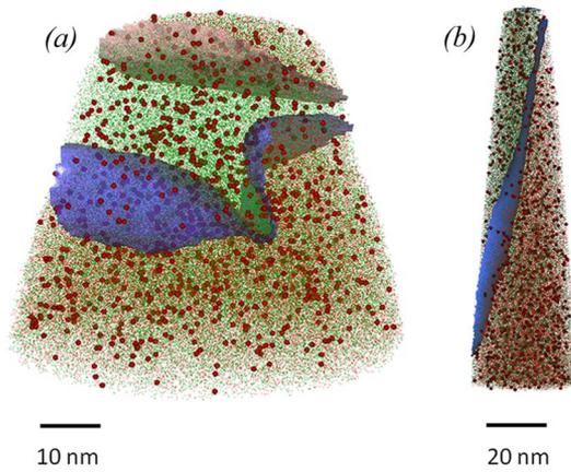
FIG. 1. (Color online) A 3D-APT reconstruction showing the  $\gamma$ (fcc)- and  $\gamma'$ ( $L1_2$ )-phases in the (a) multicomponent and (b) ternary alloys. The phases are separated by (a) 8.2 at. % Cr and (b) 12 at. % Al isoconcentration surfaces. Both reconstructions show 3% of the Ni (green), 8% of the Al (red), and 90% of the W (large red spheres) atoms detected for clarity.
