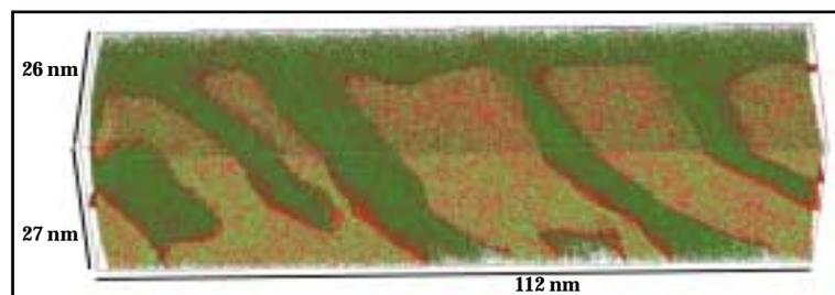
Fig. 4 — Ultrafine lamellar microstructure as determined by applying an atom map from a LEAP microscope analysis. Aluminum and titanium atoms are represented by red and green dots, respectively. The volume shown is approximately 26 × 27 × 112 nm and consists of information from 2.3 million atoms.
