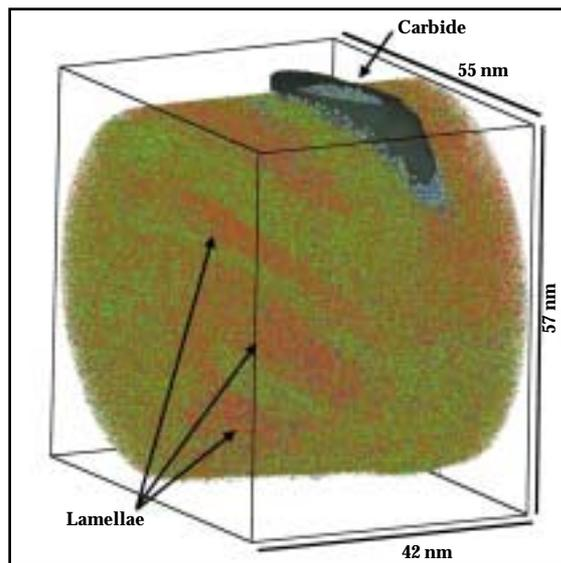
Fig. 2 — Three-dimensional atom-map obtained from a LEAP microscope analysis of a model TiAl alloy with carbide precipitates. Image displays Al atoms (red), Ti atoms (green), C atoms (grey), and O atoms (blue), with a 4.5 at.% C isoconcentration surface revealing an oxycarbide precipitate among the lamellae. The reconstruction represents a volume of 57 × 55 × 42 nm and contains 3.6 million atoms.
