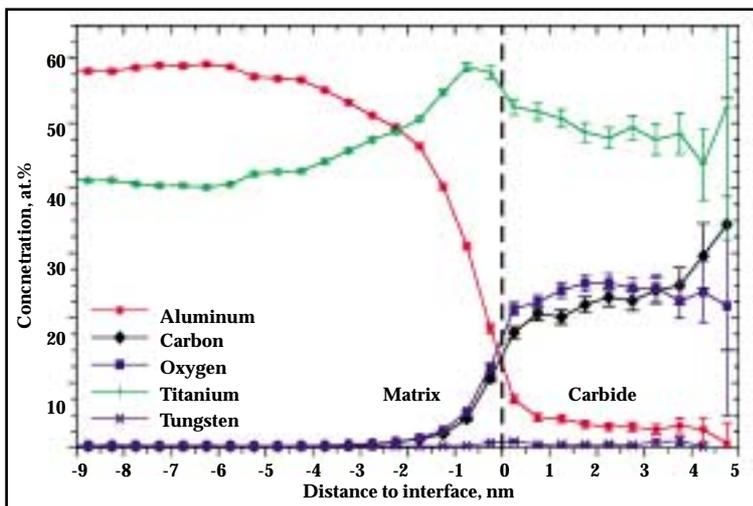
Fig. 3 — Proximity histogram of the analyzed volume shown in Figure 4 displaying concentrations with respect to a carbon isoconcentration surface (4.5 at.% C). Carbide concentration is on the right-hand side, matrix concentration is on the left-hand side of the figure. The proxigram highlights the very high oxygen concentration within the carbide.
