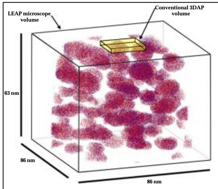
*Fig. 1 — Analysis volume collected on a specimen of a nickel-aluminum-chromium alloy in approximately one hour using the LEAP microscope, versus the volume that would be collected in the same amount of time on a conventional 3DAP (highlighted in yellow). Only Al (red) and Cr (blue) atoms within gamma-prime precipitates are shown for clarity. This image is courtesy of Chantal K. Sudbrack of Northwestern University.*
