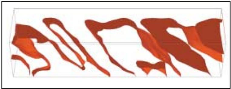
Fig. 5 — Isoconcentration surface corresponding to 51 at. % aluminum delineates fine scale lamellae with thickness ranging from 4 to 24 nm in a TiAl alloy.
