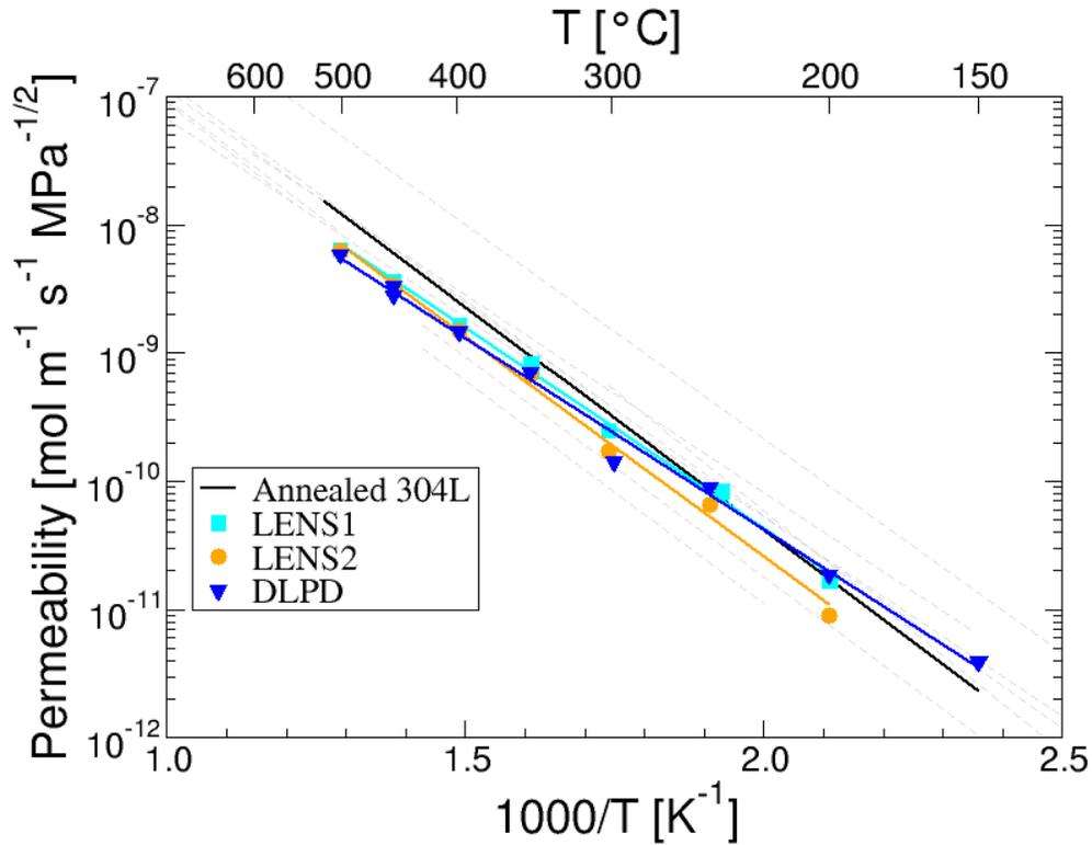
**Figure 1. Permeability of various AM steels.**
