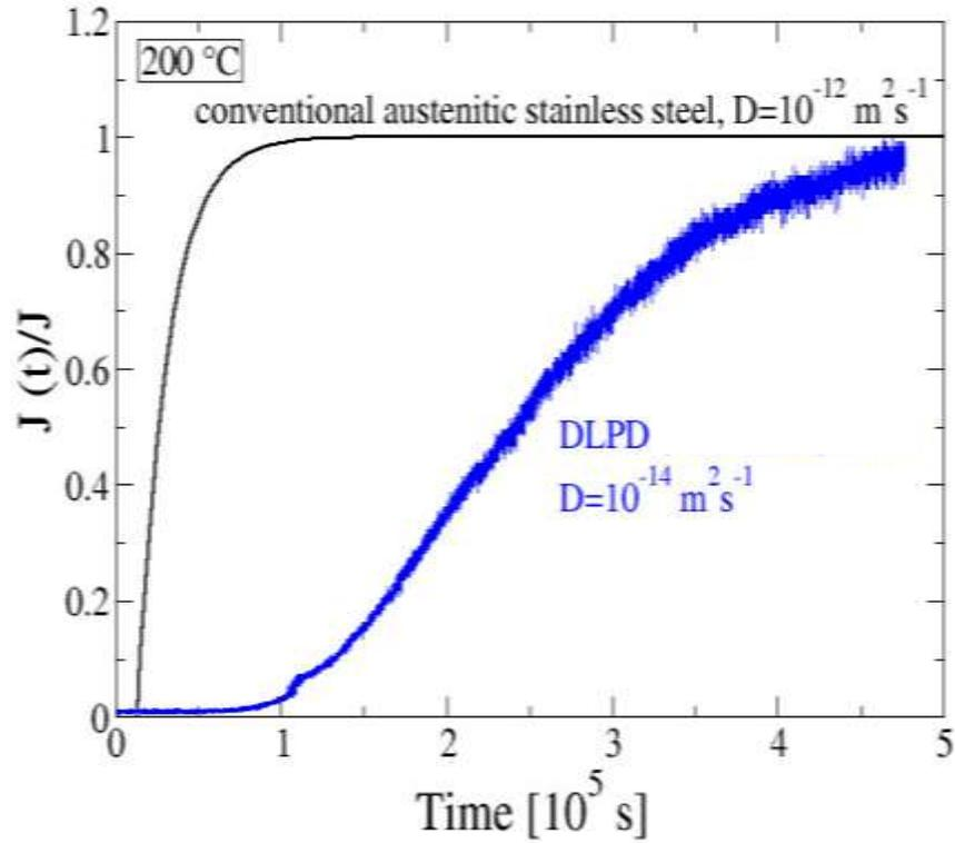
Figure 2. The permeation transient shows that it takes much longer for a DLPD steel to achieve steady-state permeation in comparison to conventional steel. This is indicative of trapping.
