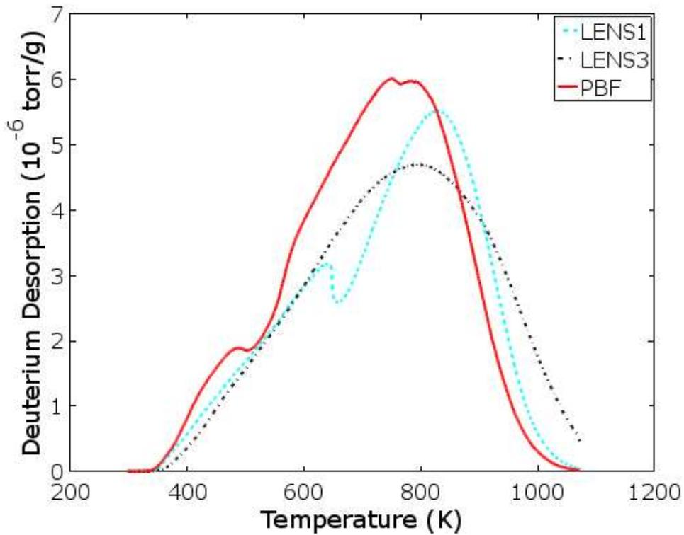
Figure 3. Thermal desorption spectra of charged samples heated  $6 \text{ }^\circ\text{C/min}$ .
