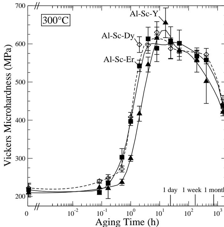
Fig. 1: Microhardness as a function of aging time at 300°C for Al-0.06 at.% Sc-0.02 at.% RE. Error bars are one standard-deviation from the mean. The three alloys exhibit similar aging responses, but Al-Sc-Y has a higher mean peak microhardness than Al-Sc-Dy, which is harder than Al-Sc-Er.
