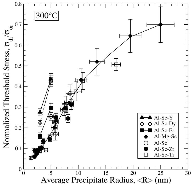
Fig. 3: Creep threshold stress, normalized by the calculated Orowan stress at 300°C, as a function of average precipitate radius,  $\langle R \rangle$ . Normalized stresses are higher for the three Al-Sc-RE microalloys than any of the previously studied Al-Sc-M alloys [5–9].
