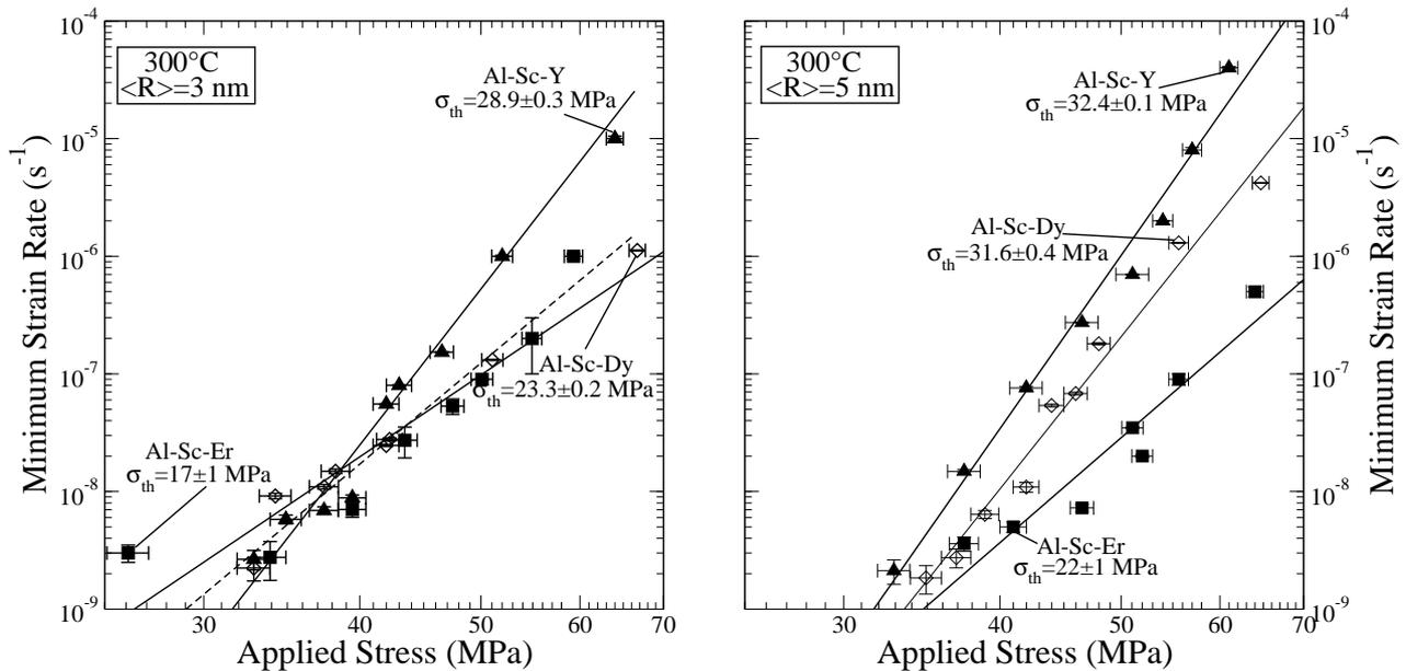
Fig. 2: Double-logarithmic plot of minimum compressive creep strain-rate vs. stress at 300°C for Al-0.06 at.% Sc-0.02 at.% RE. In the left plot, the average precipitate radius,  $\langle R \rangle = 3$  nm. In the right plot,  $\langle R \rangle = 5$  nm. For any given alloy, the specimen with the larger diameter precipitates is more creep resistant. High apparent stress exponents are indicative of a threshold stress,  $\sigma_{th}$ .
