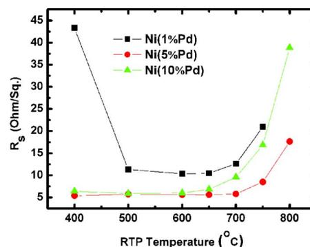
FIG. 1. (Color online) Sheet resistance measurements for  $(\text{Ni}_{1-x}\text{Pd}_x)\text{Si}/\text{Si}(100)$  thin films following rapid thermal processing for 30 s.
