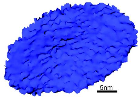
FIG. 3. (Color online) Two-dimensional projection of the three-dimensional reconstruction of the silicide-Si interface based on a Si isoconcentration surface. The root-mean-squared chemical roughness of this interface is 0.8 nm.
