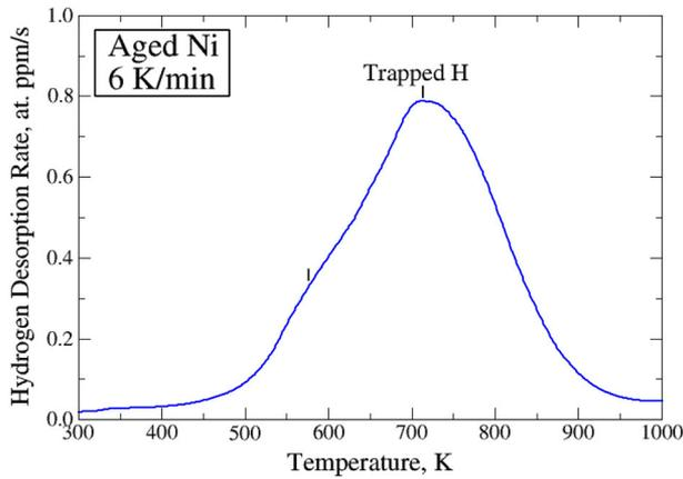
Fig. 2. Thermal desorption spectra of Ni-201 pre-charged with  $\sim 4000$  appm hydrogen then aged at room temperature for approximately 2 years, yielding  $\sim 2000$  appm hydrogen. The peak marked at ca. 700 K indicates that most of the remaining hydrogen is trapped.
