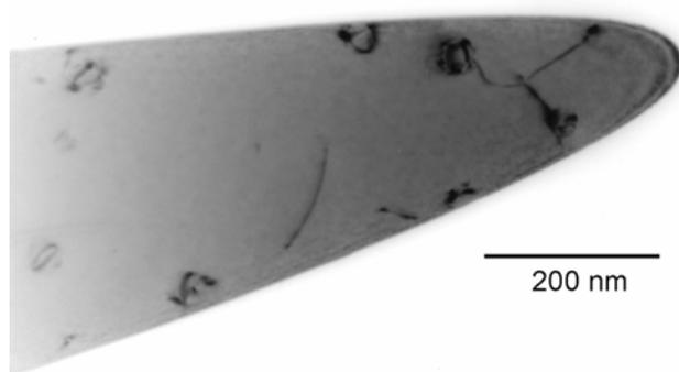
FIG. 2. Dark-field TEM image of an Al-Mg-Sc atom probe specimen containing semi-coherent Al<sub>3</sub>Sc precipitates.
