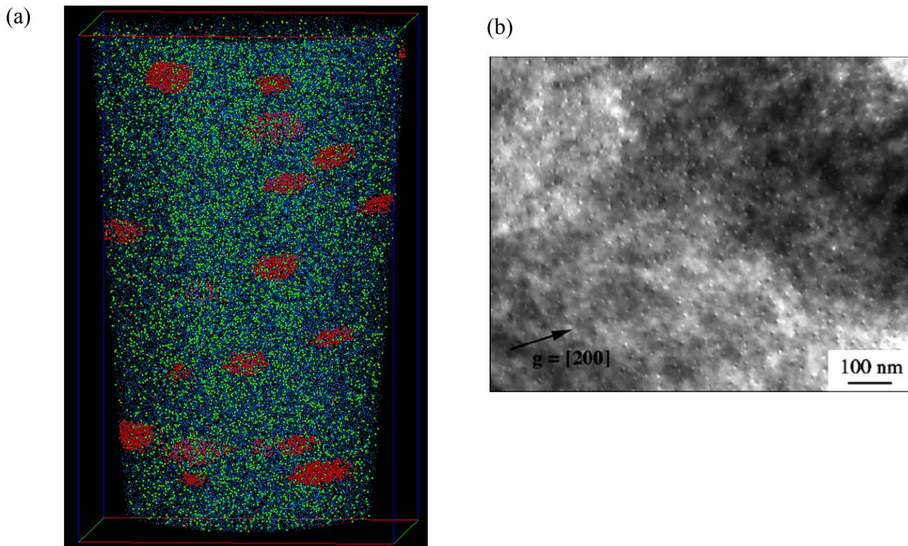
FIG. 1. Al–2.2 at.% Mg–0.12 at.% Sc alloy after aging at 300°C for 24 h: (a) 3DAP reconstruction showing Al<sub>3</sub>Sc precipitates. Al atoms are represented in blue, Mg in green and Sc atoms in red. The volume is 54nm x 54nm x 89nm. (b) CTEM micrograph showing a high number density of Al<sub>3</sub>Sc precipitates: dark-field image, exhibiting Ashby–Brown strain coherency contrast, obtained with a [200] reflection.
