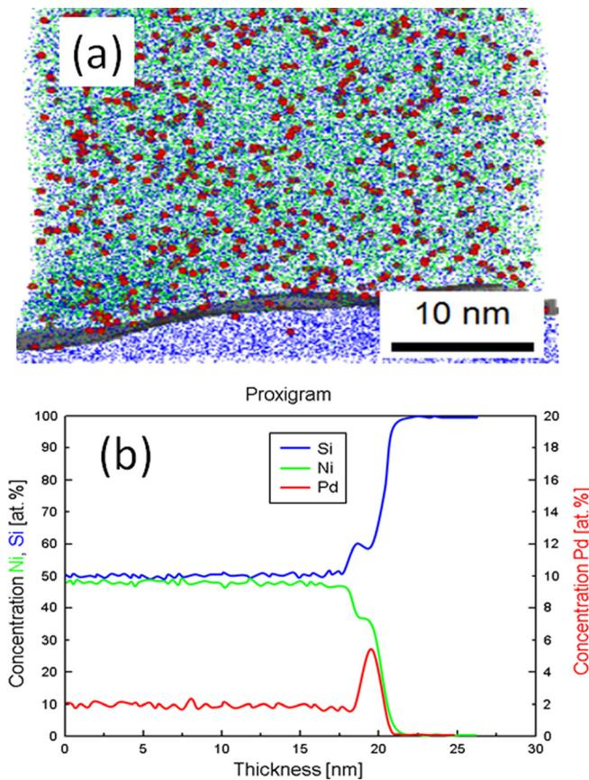
FIG. 1. (Color online) (a) Two-dimensional projection of the full three-dimensional reconstruction of LEAP tomography data showing the distribution of elements and the isoconcentration surface (shaded sheet) that defines the heterophase interface. (b) Proximity histogram displaying the concentrations of Ni, Si, and Pd versus film-depth. Concentrations were calculated for a series of isoconcentration surfaces moving into the thin film.
