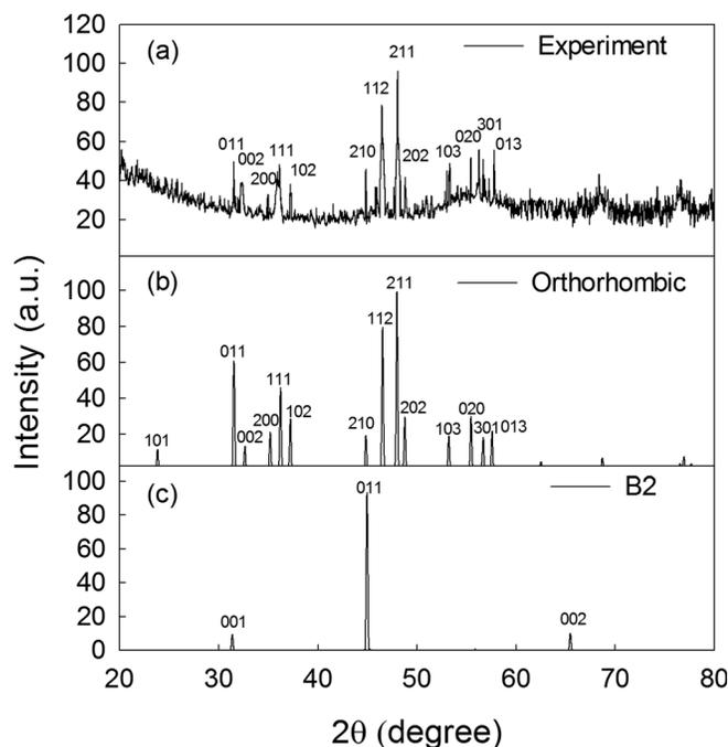
FIG. 2. X-ray diffraction spectra of NiSi: (a) experimentally determined; (b) calculated NiSi orthorhombic structure; and (c) calculated NiSi(B2) structure.
