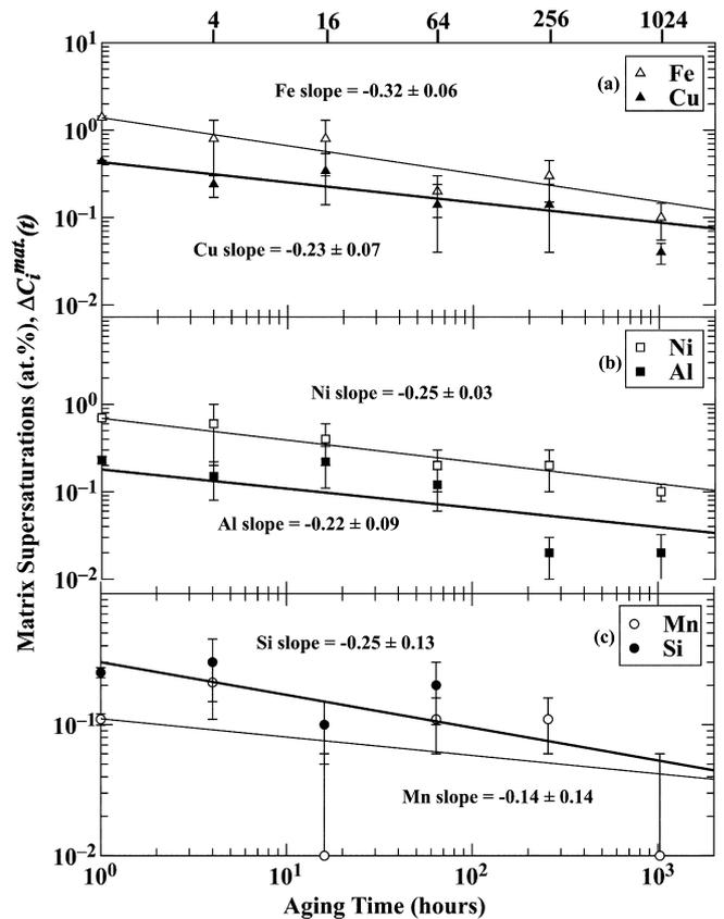
Fig. 10. Double logarithmic plots of matrix supersaturations,  $\Delta C_i^{\text{mat.}}(t)$ , as a function of aging time, when aged at 500 °C, for (a) Cu and Fe; (b) Ni and Al; and (c) Mn and Si. The slopes of the plots yield the coarsening time exponents for each element.
