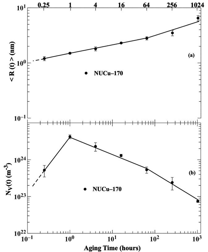
Fig. 6. The (a) mean precipitate radius,  $\langle R(t) \rangle$ ; and (b) number density,  $N_V(t)$ , as a function of aging time for an aging temperature of 500 °C.
