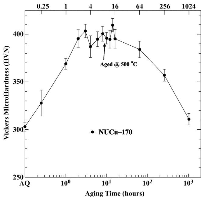
Fig. 1. Vickers microhardness (VHN) as a function of aging time (h) when the NUCu-170 steel is aged at 500 °C. A plateau of ~395 VHN is seen between 2 and 16 h.
