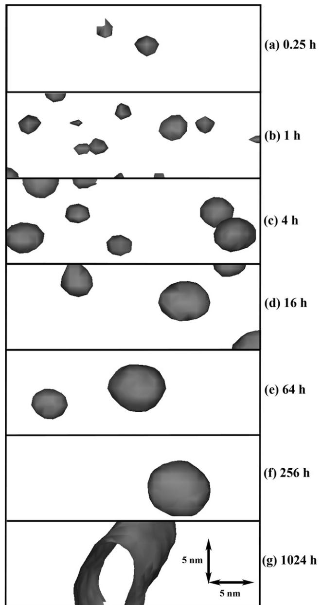
Fig. 2. Copper-rich precipitates as delineated by 10 at.% Cu isoconcentration surfaces, when the steel is aged at 500 °C for: (a) 0.25 h; (b) 1 h; (c) 4 h; (d) 16 h; (e) 64 h; (f) 256 h; (g) 1024 h. Each reconstruction,  $10 \times 10 \times 30 \text{ nm}^3$  ( $3000 \text{ nm}^3$ ), is a subset of an analyzed volume and contains approximately 130,000 atoms.
