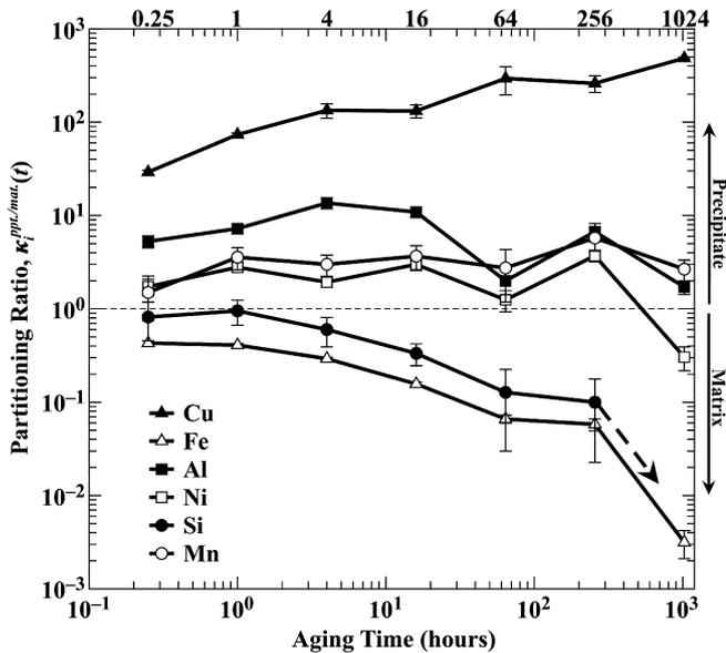
Fig. 9. Partitioning ratios,  $\kappa_i^{\text{ppt./mat.}}(t)$ , of the concentrated multicomponent Fe–Cu steel as a function of aging time, when aged at 500 °C, from 0.25 to 1024 h. The horizontal dashed line indicates the division between the precipitate and matrix phases. The dashed arrow for the Si ratio represents the zero Si concentration within the precipitate at 1024 h.
