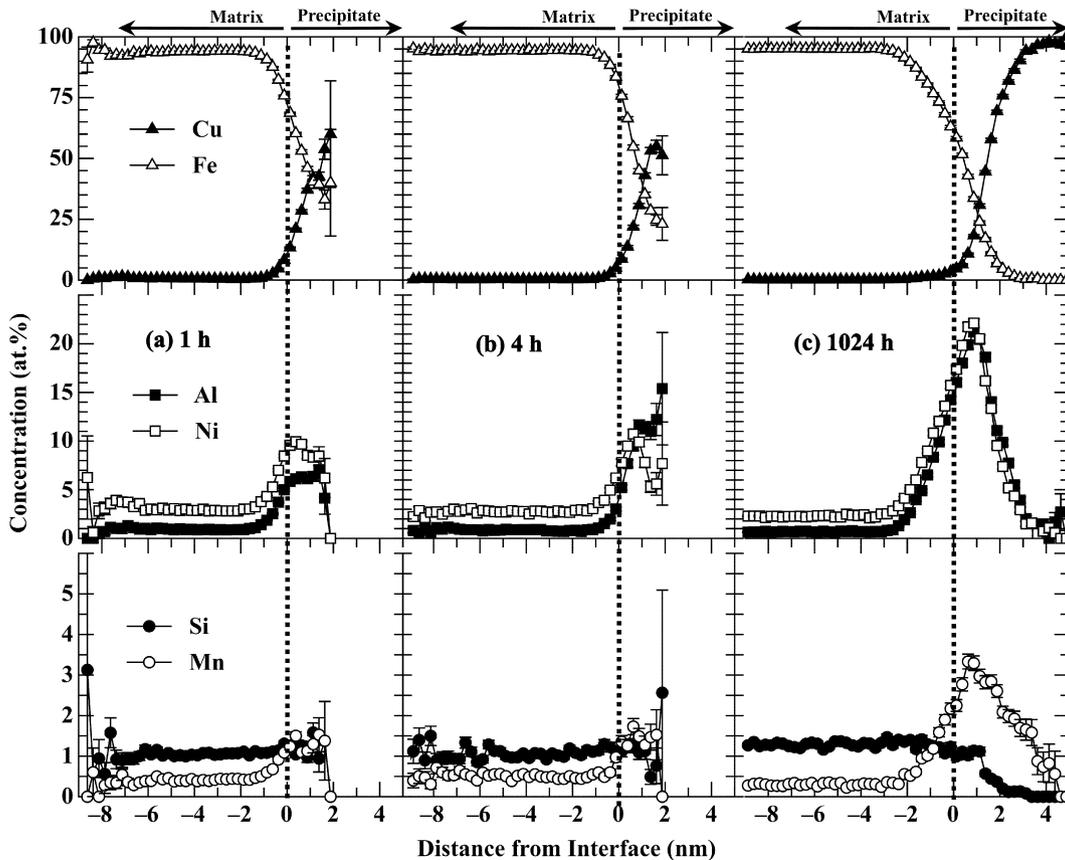
Fig. 8. Proxigram concentration profiles (at.%) for Cu, Fe, Ni, Al, Si and Mn, when the steel is aged at 500 °C, for (a) 1 h, (b) 4 h and (c) 1024 h. The dotted vertical lines indicate the  $\alpha$ -Fe matrix/precipitate heterophase interface.
