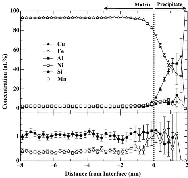
Fig. 7. Proxigram concentration profiles (at.%) for Cu, Fe, Al, Si and Mn, when the steel is aged at 500 °C for 0.25 h. The dotted vertical line corresponds to the  $\alpha$ -Fe matrix/precipitate heterophase interface.
