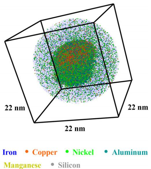
Fig. 4. Three-dimensional atom-probe tomographic reconstruction of a spheroidal shaped precipitate found in the 1024 h aged condition. The Cu, Ni, Al and Mn atoms are shown as spheres (not to scale) allowing visualization of the precipitates and heterophase interfaces. Only 20% of the Fe and 50% of the Cu, Ni, Al and Mn atoms are shown for clarity.
