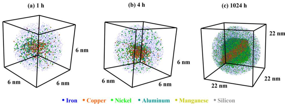
Fig. 3. Three-dimensional atom-probe tomographic reconstructions of representative precipitates in the (a) 1 h, (b) 4 h and (c) 1024 h aged conditions. The precipitate presented in (c) is of rod-like morphology. The Cu, Ni, Al and Mn atoms are shown as spheres (not to scale), allowing visualization of the precipitates and heterophase interfaces. Only 20% of the Fe and 50% of the Cu, Ni, Al, and Mn atoms are shown in (c) for clarity.
