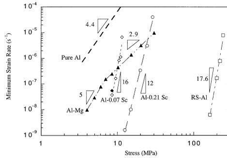
Figure 3. Minimum creep rate of Al(Sc) alloys at 300°C as a function of applied stress. Data for coarse-grained pure Al at 300°C (15), Al-2 wt.% Mg at 300°C (18), and RS-Al (Al-11.7 wt.% Fe-1.15 wt.% V-2.4 wt.% Si) at 314°C in compression (19) are presented for comparison.
