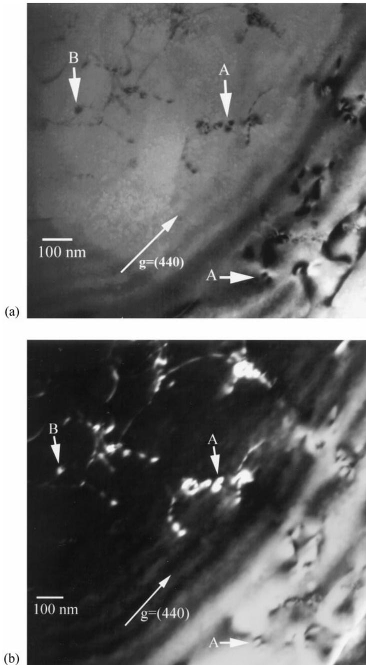
Figure 1. Bright-field (a) and dark-field (b) two-beam TEM micrographs, recorded employing a 440 operating reflection, of a crept Al-0.07 wt.% Sc tested at 300°C and cooled under load. Arrows on micrographs denote the presence of Al<sub>3</sub>Sc precipitates with strain-field contrast (A) and an Al<sub>3</sub>Sc precipitate interacting with a dislocation (B).
