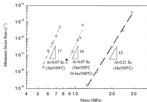
Figure 2. Minimum creep rate of Al(Sc) alloys at 300°C as a function of applied tensile stress (aging time and temperature are given in parentheses). Second data point (◆) for Al-0.07 wt.% Sc was used for verification of aging characteristics.
