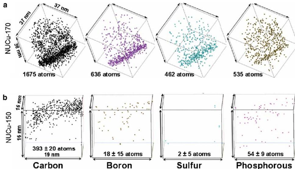
**Figure 6.** 3D APT atom-by-atom reconstructions of grain boundaries in (a) NUCu-170 steel and (b) NUCu-150 (1st heat) steel, displaying the distribution of carbon, boron, sulfur, and phosphorous atoms. Carbon is strongly segregated at grain boundaries in both steels. The alloy with the lower fracture toughness, NUCu-170, however, exhibits significantly higher levels of boron, sulfur, and phosphorous segregation.
