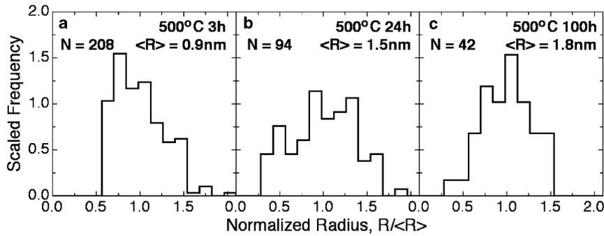
**Figure 5.** Particle size distributions of the homogeneously distributed copper-rich precipitates in NUCu-150 (1st heat) steel, after aging at 500 °C for (a) 3 h; (b) 24 h; or (c) 100 h.
