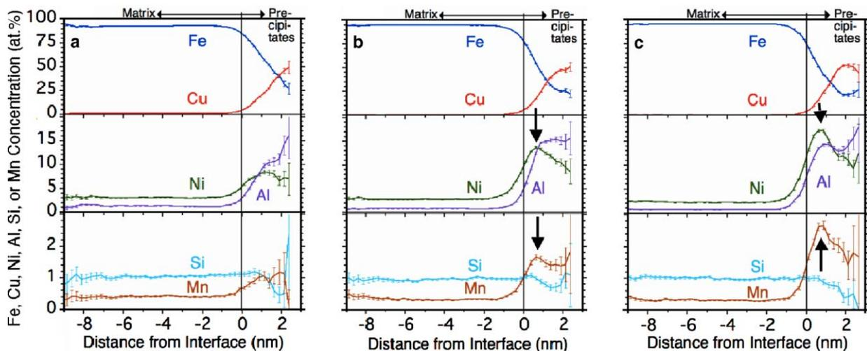
**Figure 4.** Proxigram concentration profiles for copper-rich precipitates in the NUCu-150 (1st heat) steel after aging at 500 °C for (a) 3 h; (b) 24 h; or (c) 100 h. The maximum copper concentration in the precipitates' centers remains at about 50% for aging times up to 100 h. The precipitates, however, develop a spherical shell enriched in Ni and Mn (black arrows). The error bars are the statistical uncertainty,  $\sigma = \sqrt{c(1-c)/N}$  for a concentration  $c$  and  $N$  total atoms.
