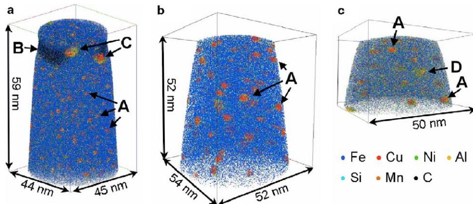
**Figure 2.** Three-dimensional atom-by-atom atom-probe tomographic reconstructions of specimen volumes in a NUCu-150 (1st heat) steel after aging at 500 °C for (a) 3 h; (b) 24 h; or (c) 100 h, illustrating the temporal evolution of the copper-rich precipitates used for precipitation strengthening of this HSLC steel. The reconstructed volumes contain (a) 3.0 million atoms; (b) 3.3 million atoms; and (c) 2.6 million atoms.
