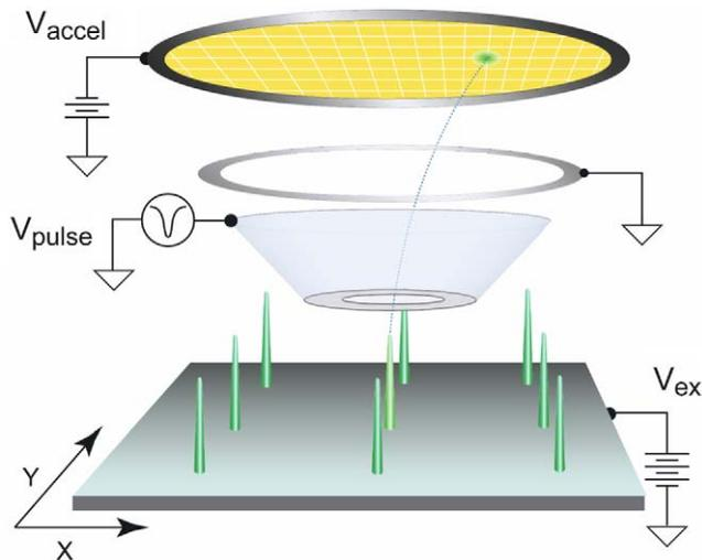
**Figure 1.** A schematic of a LEAP tomograph scanning a planar array of microtips using a high-voltage pulsed electric field. Also shown schematically is the variable voltage post-evaporation (secondary) accelerator,  $V_{\text{accel}}$ . Courtesy of Prof. Lincoln Lauhon, Northwestern University.
