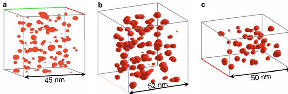
**Figure 3.** The copper-rich precipitates in the NUCu-150 (1st heat) steel are discernible more clearly after discriminating with an isoconcentration surface at a 5 at.% copper threshold level, after aging for (a) 3 h; (b) 24 h; or (c) 100 h.
