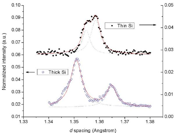
FIG. 2. (Color online) Time focused Si 004 reflection data obtained on SMARTS from the complete  $2\theta = +90^\circ$  bank (bank 1) detectors for the 20 and 0.7 mm thick Si samples.
