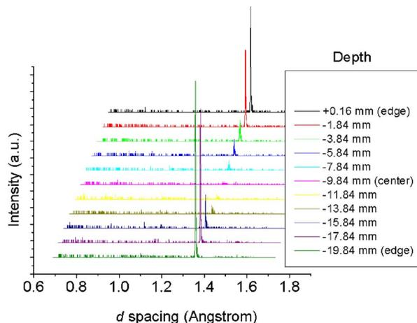
FIG. 3. (Color online) Results of the depth scan on ENGIN X of the 20 mm thick Si specimen. The data were collected in one detector element at  $2\theta = -88.43^\circ$ . The Si 004 peak intensity is seen to exist near each sample edge, yet it disappears at the sample center.
